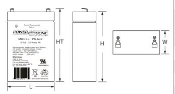
**W**: 1.30 (33) **H**: 4.65 (118) **HT**: 4.80 (122) **L**: 2.60 (66) Tolerances are +/- 0.04 in. (+/- 1mm) and +/- 0.08 in. (+/- 2mm) for height dimensions. All data subject to change without notice.
